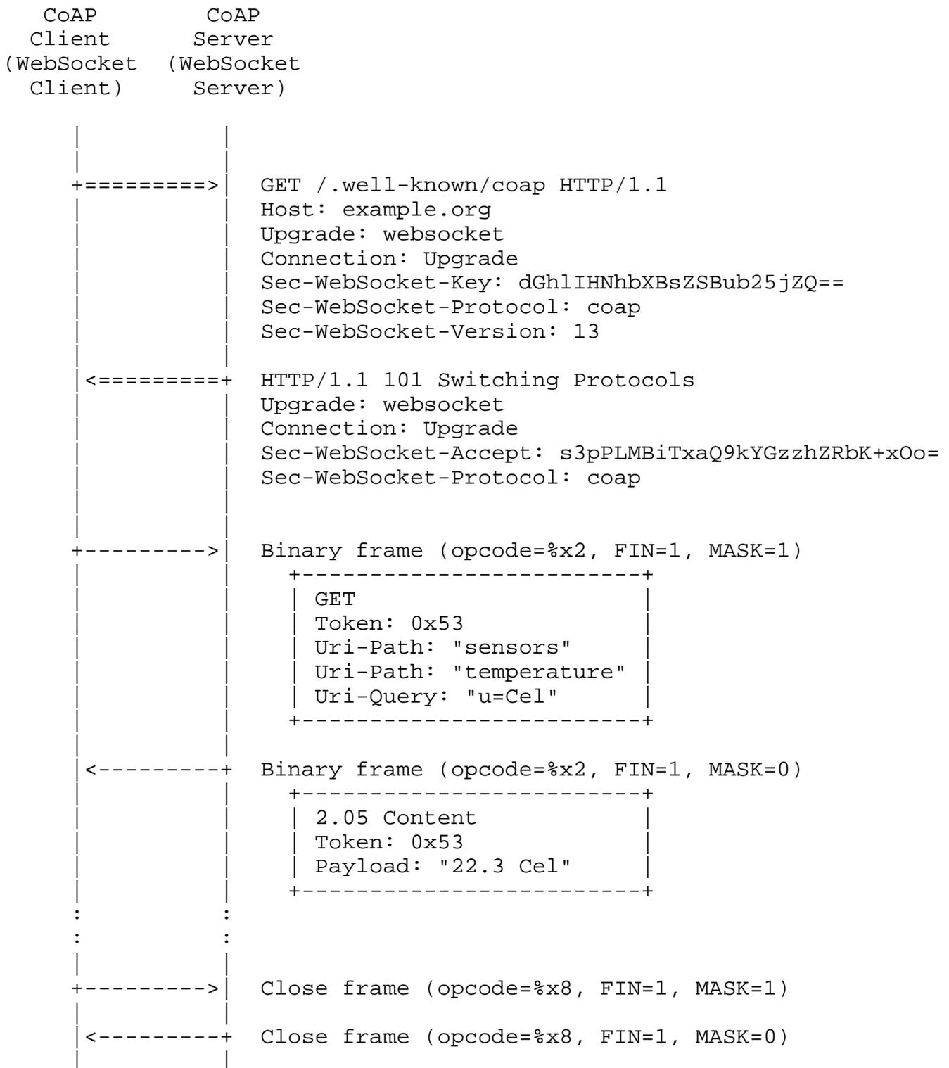
Figure 19: A CoAP client retrieves the representation of a resource identified by a "coap+ws" URI
