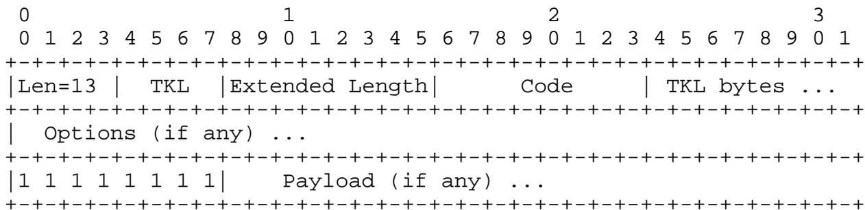
Figure 4: CoAP frame with 8-bit Extended Length field.
