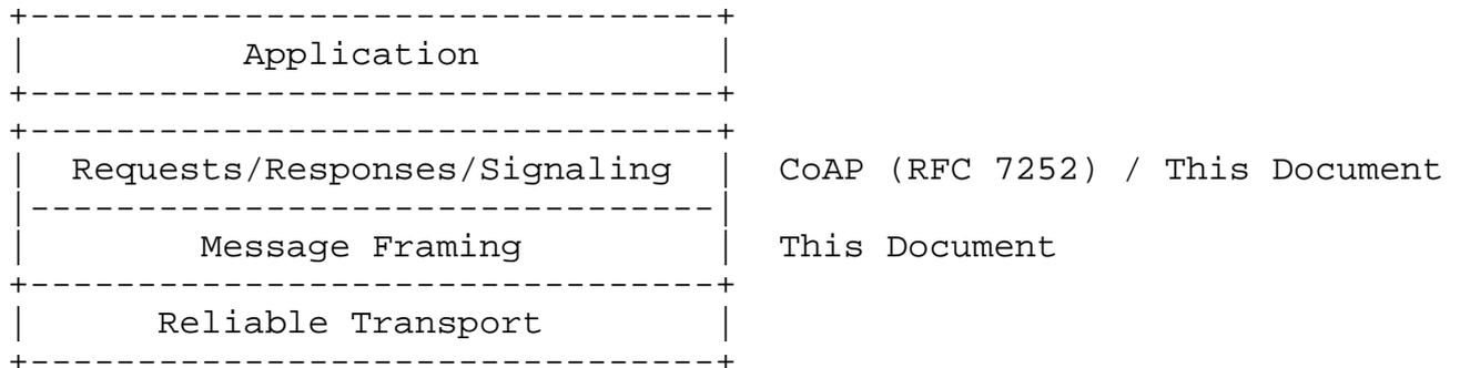
Figure 1: Layering of CoAP over Reliable Transports
