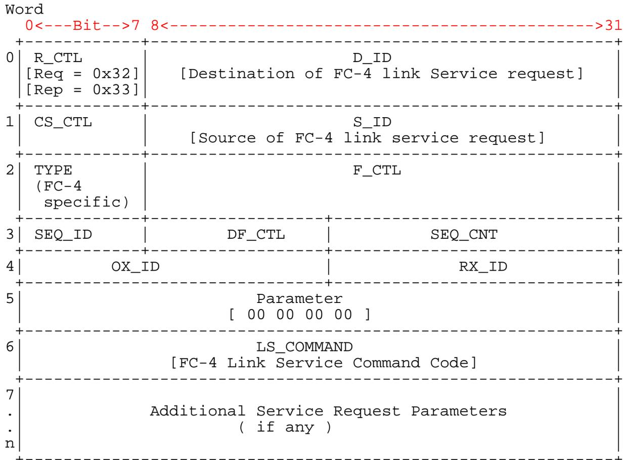
Figure 20 -- Format of an FC-4 Link Service Frame
