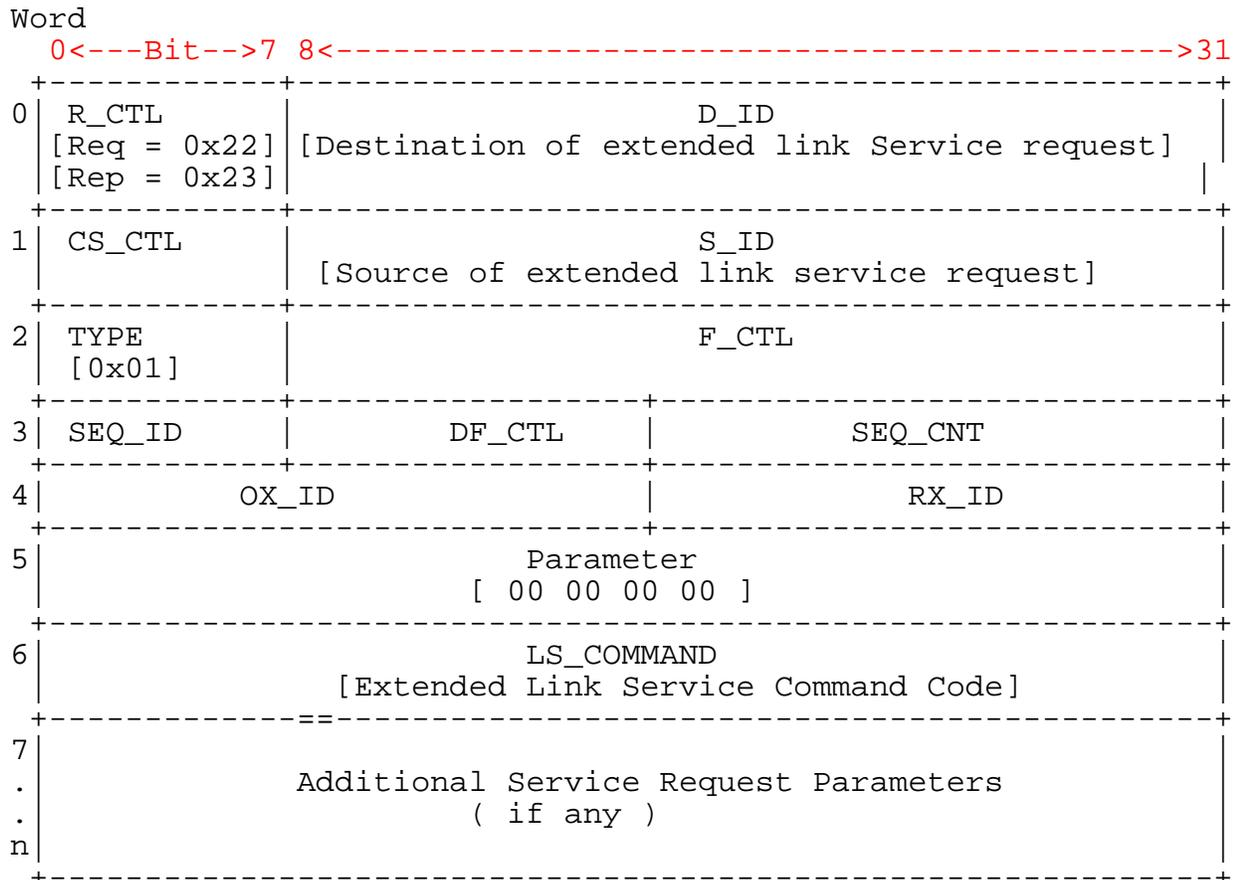
Figure 19 -- Format of an Extended Link Service Frame
