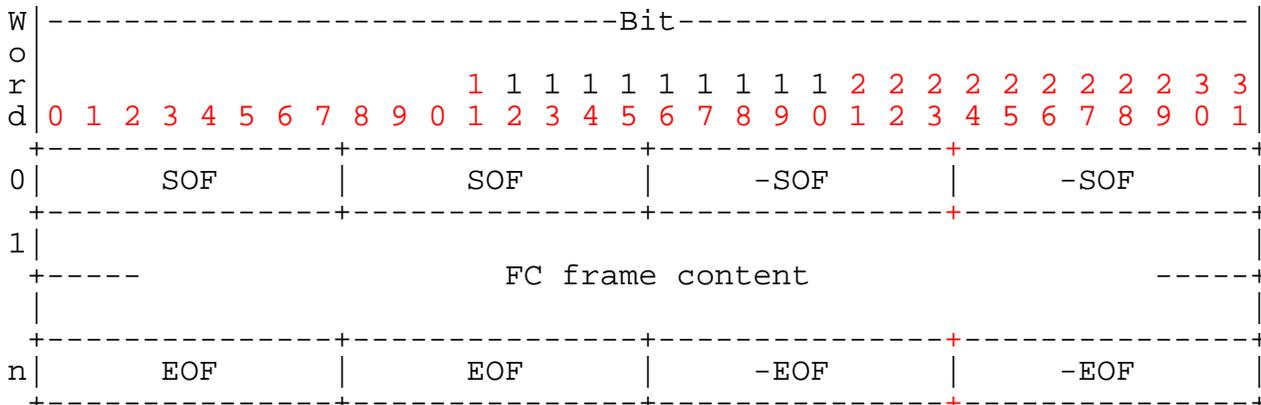
Figure 17 -- FC Frame Encapsulation Format
