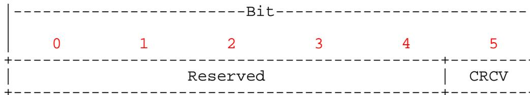
Figure 16 -- iFCP Common Encapsulation Flags
