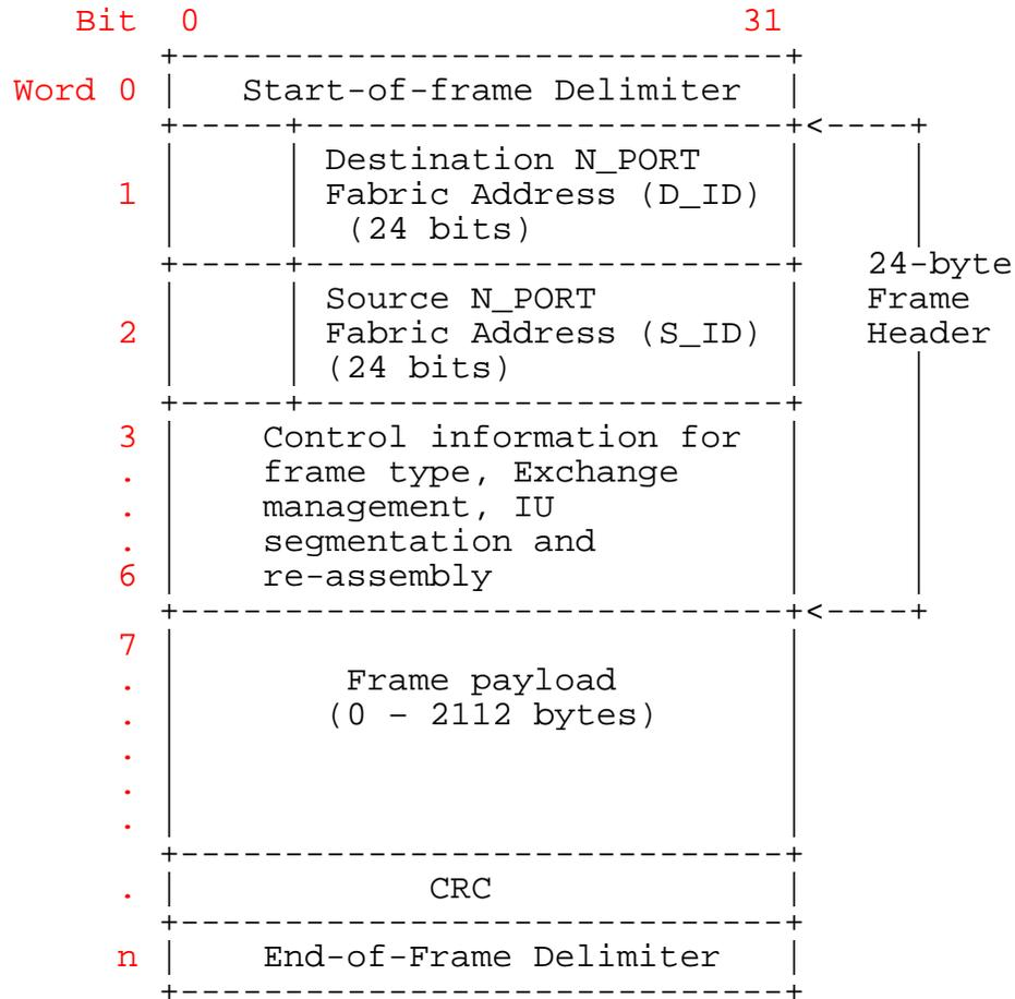
Figure 4 -- Fibre Channel Frame Format
