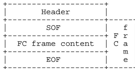
Figure 13 -- Encapsulation Format
