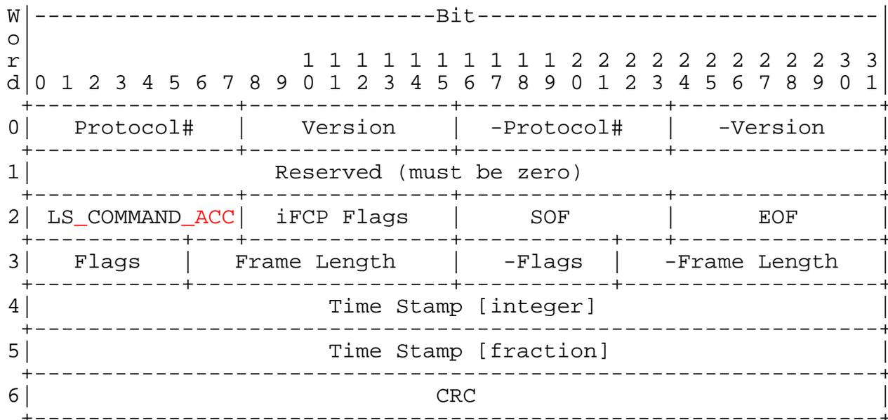
Figure 14 --- Encapsulation Header Format
