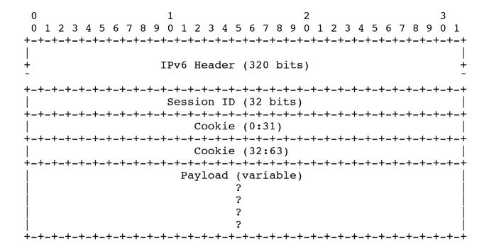
The combined IPv6 and Keyed IP Tunnel header contains the following fields:
