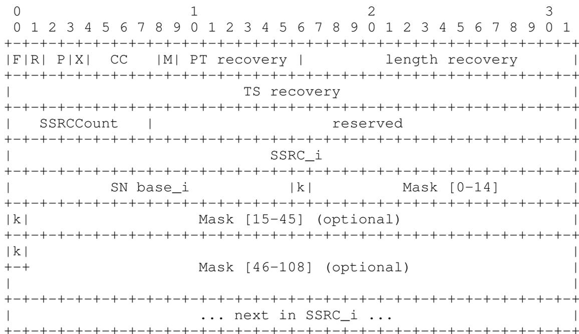
Figure 10: Format of the FEC header
