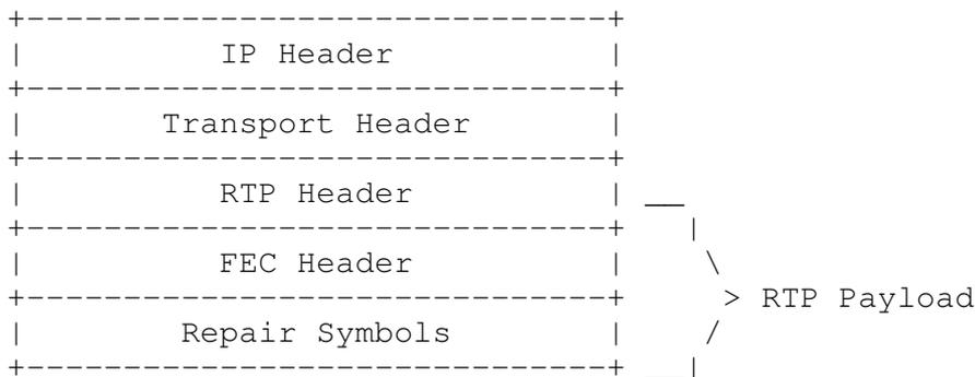
Figure 9: Format of repair packets
