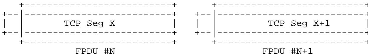
Figure 11: Aligned FPDU placed immediately after TCP header
