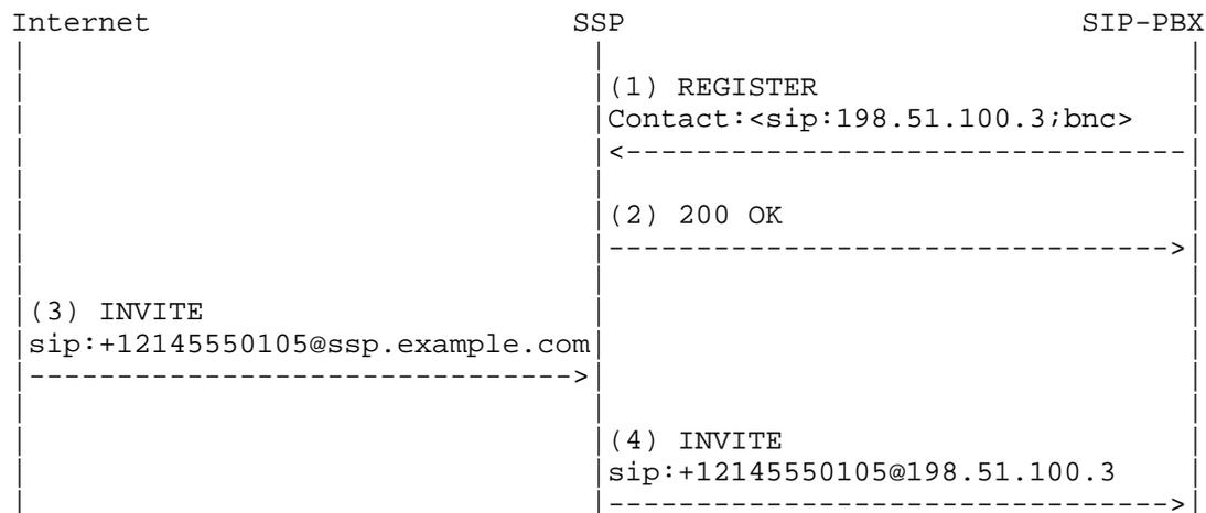
(1) The SIP-PBX registers with the SSP for a range of AORs.
