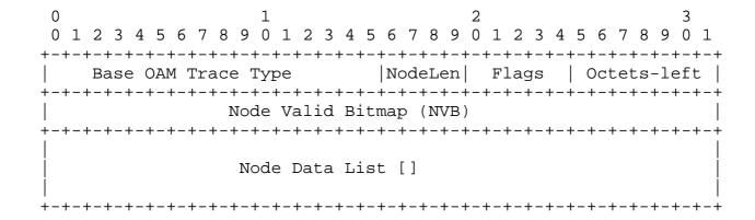
Figure 1: iOAM Header Format with Node Valid Bitmap (NVB)
