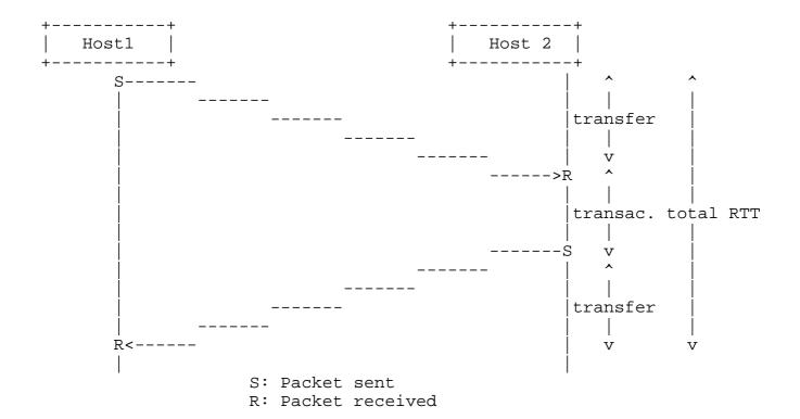
Figure 1 illustrates these delays. The labeled times (S and R) designate the times in which the packet is sent and received, respectively, by the network interface.
