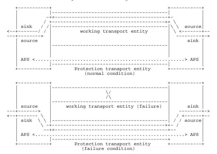
Figure 3 1:1 Bidirectional Linear Protection Switching
