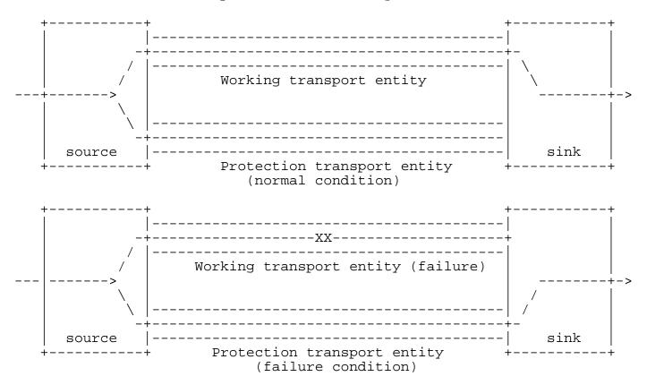
Figure 1 1+1 Unidirectional Linear Protection Switching
