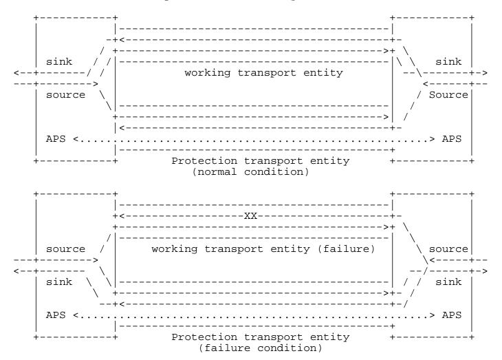
Figure 2 1+1 Bidirectional Linear Protection Switching
