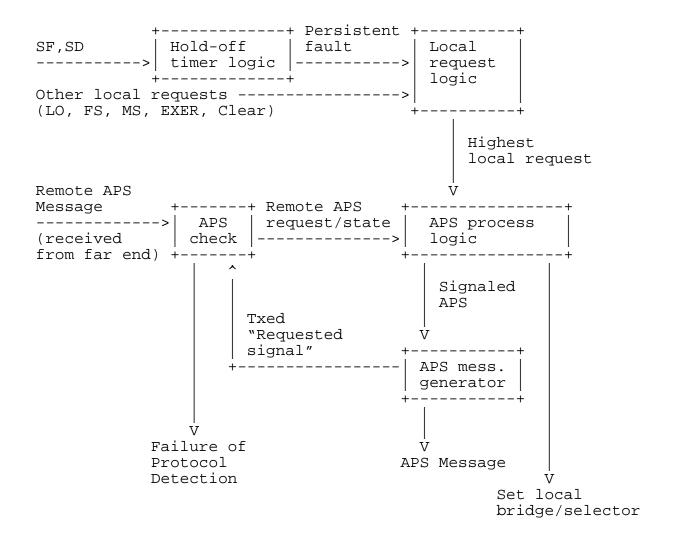
Figure 7 Protection Switching Logic
