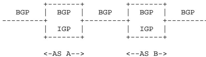
This diagram points out that, while BGP alone carries information between AS's, both BGP and an IGP may carry information across an AS. Ensuring consistency of routing information between BGP and an IGP within an AS is a significant issue and is discussed at length later in Appendix A.
