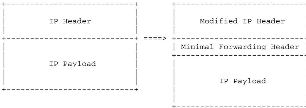
The IP header of the original datagram is modified, and the minimal forwarding header is inserted into the datagram after the IP header, followed by the unmodified IP payload of the original datagram (e.g., transport header and transport data). No additional IP header is added to the datagram.
