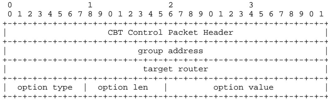
Figure 4. JOIN\_ACK Packet Format
