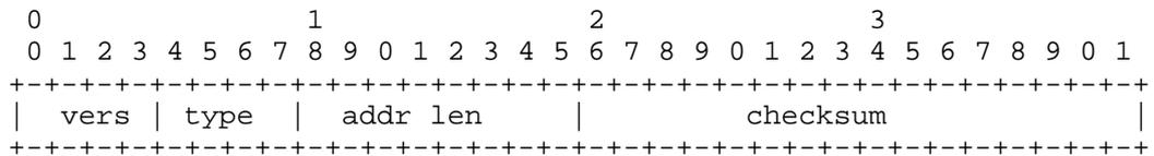
Figure 1. CBT Common Control Packet Header
