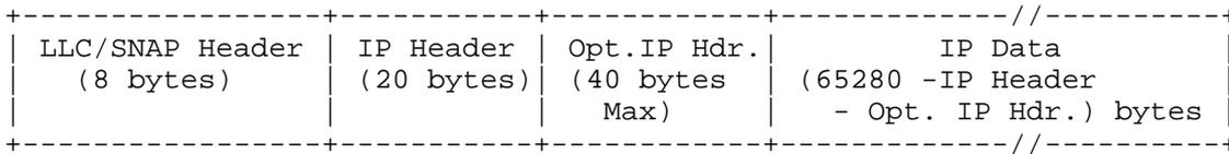
Fig. 4 Format of FC Sequence Payload carrying IP
