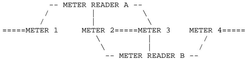
Several uniquely identified meters may report to one or more meter readers. The diagram above gives an example of how multiple meters and meter readers could be used.
