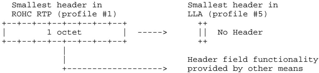
The fields present in the ROHC RTP headers for U/O-mode PT0 are the packet type identifier, the sequence number and the CRC. The subsequent sections elaborate more on how the functionality of these fields is replaced for NHP.
