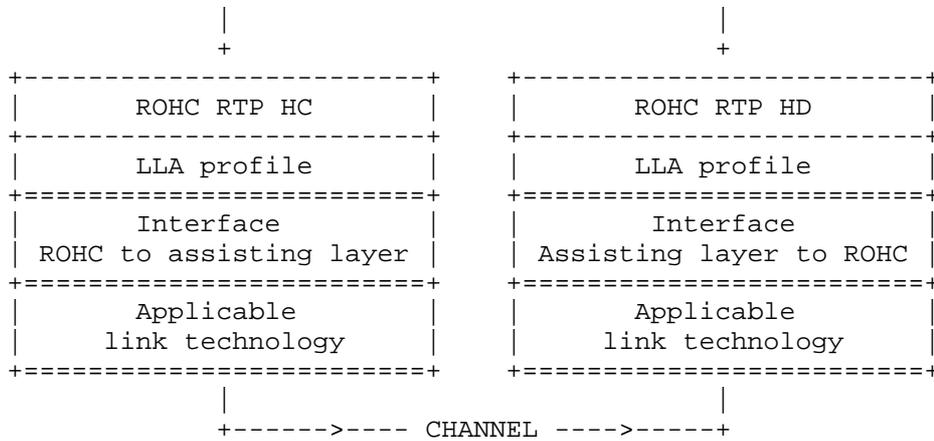
The figure above shows the various levels, as defined in [ROHC] and this document, constituting a complete implementation of the LLA profile. The figure also underlines the need for additional documents to specify how to implement these interfaces for a link technology for which this profile is relevant.
