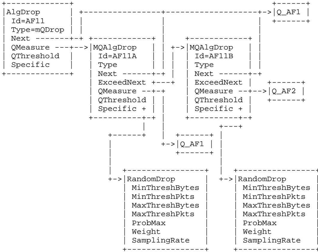
Figure 8: Multiple Queue Random Dropper Usage Example
