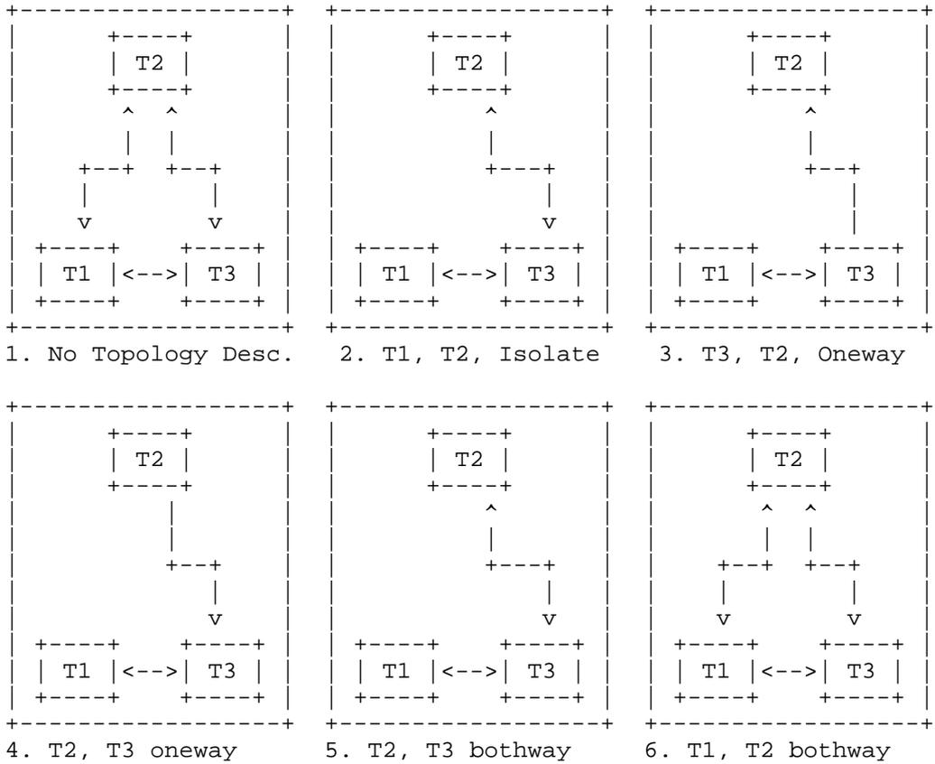
Note: the direction of the arrow indicates the direction of flow.
