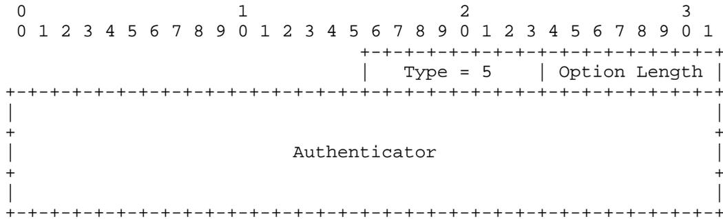
The Binding Authorization Data option is valid in the Binding Update and Binding Acknowledgement.
