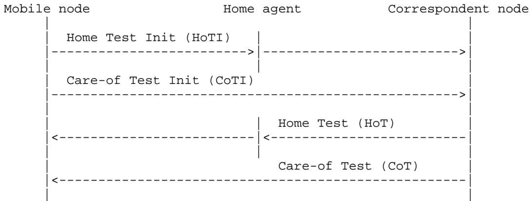
The Home and Care-of Test Init messages are sent at the same time. The procedure requires very little processing at the correspondent node, and the Home and Care-of Test messages can be returned quickly, perhaps nearly simultaneously. These four messages form the return routability procedure.
