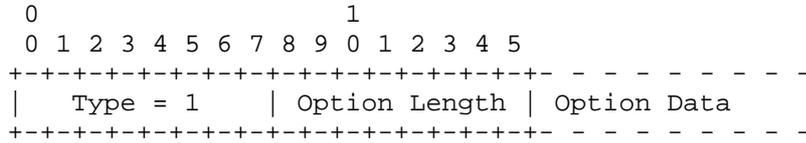
The PadN option is used to insert two or more octets of padding in the Mobility Options area of a mobility message. For N octets of padding, the Option Length field contains the value N-2, and the Option Data consists of N-2 zero-valued octets. PadN Option data MUST be ignored by the receiver.
