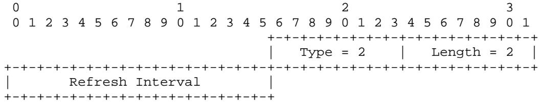
The Binding Refresh Advice option is only valid in the Binding Acknowledgement, and only on Binding Acknowledgements sent from the mobile node's home agent in reply to a home registration. The Refresh Interval is measured in units of four seconds, and indicates remaining time until the mobile node SHOULD send a new home registration to the home agent. The Refresh Interval MUST be set to indicate a smaller time interval than the Lifetime value of the Binding Acknowledgement.
