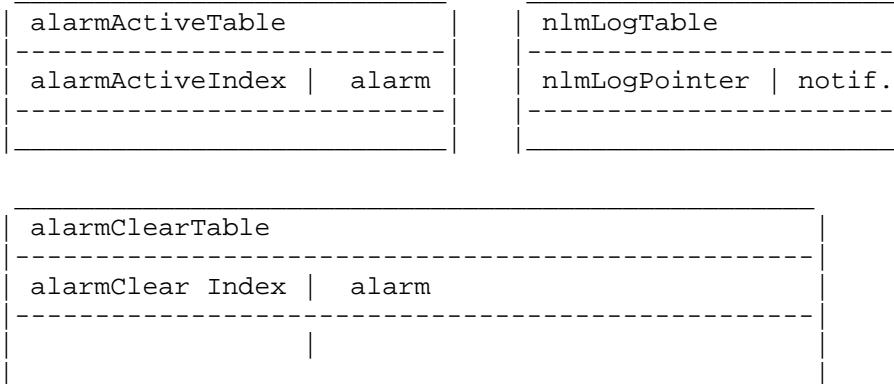
1. Some time later, a link goes down generating a linkDown Notification, which is sent out and logged in the Notification Log. As this Notification is modelled as an alarm state, an entry is added to the active alarm table.
