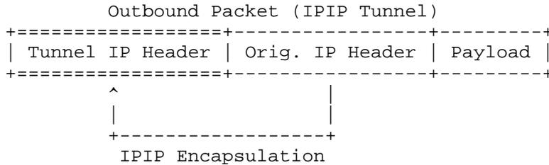
Figure 4: Outbound Packet Construction for IPIP Tunnel
