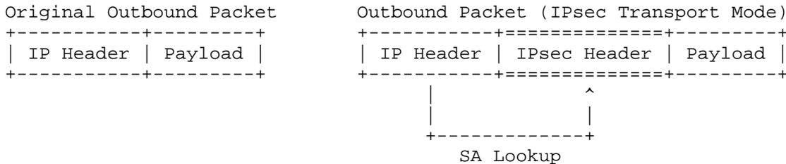
Figure 1: Outbound Packet Construction under IPsec Transport Mode
