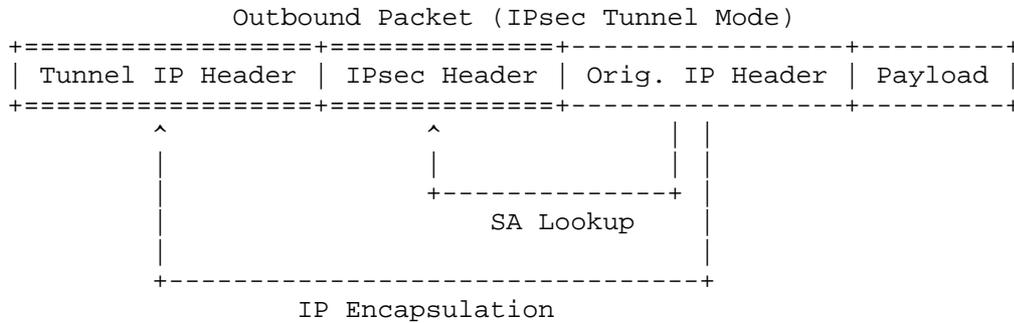
Figure 2: Outbound Packet Construction under IPsec Tunnel Mode
