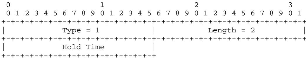
Hold Time is the number of seconds a receiver MUST keep the neighbor reachable. If the Hold Time is set to '0xffff', the receiver of this message never times out the neighbor. This may be used with dial-on-demand links to avoid keeping the link up with periodic Hello messages. Furthermore, if the Holdtime is set to '0', the information is timed out immediately. The Hello Hold Time option MUST be used by PIM-DM routers.
