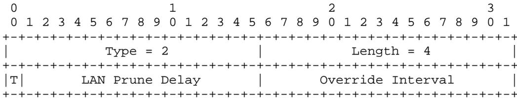
The LAN\_Prune\_Delay option is used to tune the prune propagation delay on multi-access LANs. The T bit is used by PIM-SM and SHOULD be set to 0 by PIM-DM routers and ignored upon receipt. The LAN Delay and Override Interval fields are time intervals in units of milliseconds and are used to tune the value of the J/P Override Interval and its derived timer values. Section 4.3.5 describes how these values affect the behavior of a router. The LAN Prune Delay SHOULD be used by PIM-DM routers.
