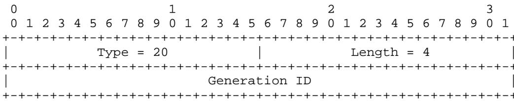
Generation ID is a random value for the interface on which the Hello message is sent. The Generation ID is regenerated whenever PIM forwarding is started or restarted on the interface. The Generation ID option MAY be used by PIM-DM routers.
