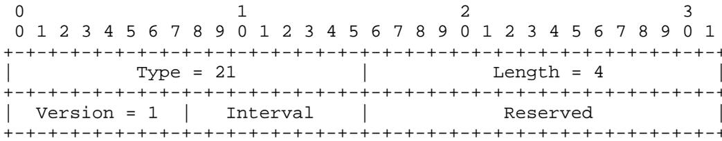
The Interval field is the router's configured State Refresh Interval in seconds. The Reserved field is set to zero and ignored upon receipt. The State Refresh Capable option MUST be used by State Refresh capable PIM-DM routers.
