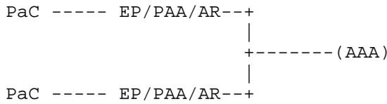
Figure 3: PAA co-located with EP and AR.
