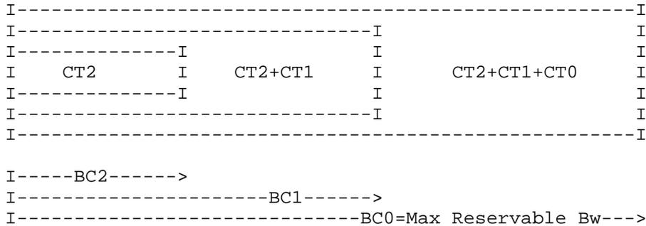
While simpler Bandwidth Constraints models or, conversely, more flexible/sophisticated Bandwidth Constraints models can be defined, the Russian Dolls Model is attractive in some DS-TE environments for the following reasons:
