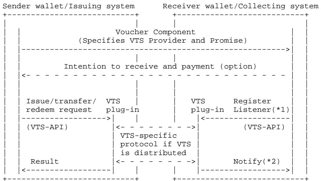
(\*1) Registration is optional. Note also that the VTS plug-ins are usually pre-registered when the wallet or collecting system is started.
