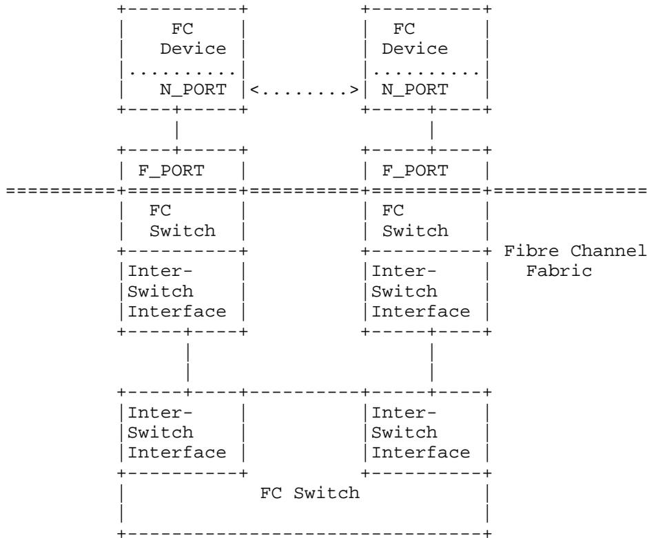
Figure 2. Multi-Switch Fibre Channel Fabric
