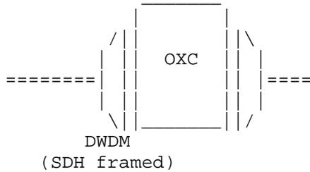
A TE link is a group of one or more of the interfaces on the OXC. All lambdas associated with a particular interface are required to have identifiers unique to that interface, and these identifiers are used as labels (see 3.2.1.1 of [GMPLS-SIG]).
