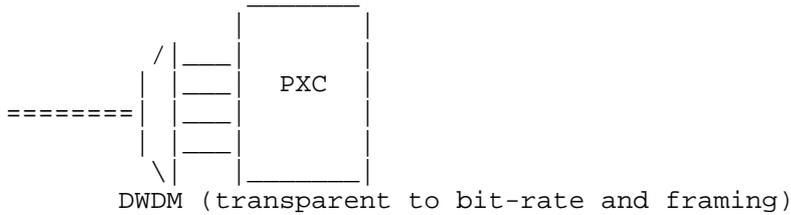
A TE link is a group of one or more interfaces on the PXC. All interfaces on a given PXC are required to have identifiers unique to that PXC, and these identifiers are used as labels (see 3.2.1.1 of [GMPLS-SIG]).
