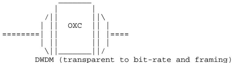
A TE link is a group of one or more of the interfaces on the OXC. All lambdas associated with a particular interface are required to have identifiers unique to that interface, and these identifiers are used as labels (see 3.2.1.1 of [GMPLS-SIG]).
