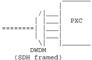
A TE link is a group of one or more interfaces on the PXC. All interfaces on a given PXC are required to have identifiers unique to that PXC, and these identifiers are used as labels (see 3.2.1.1 of [GMPLS-SIG]).
