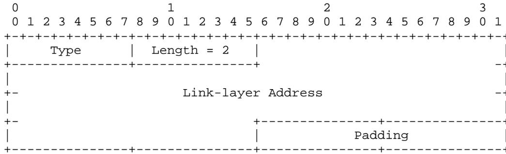
Figure 23: Source/Target Link-layer Address Option for Fibre Channel
