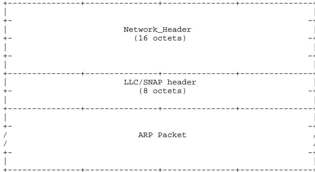
Figure 4: FC Information Unit Mapping an ARP Packet
