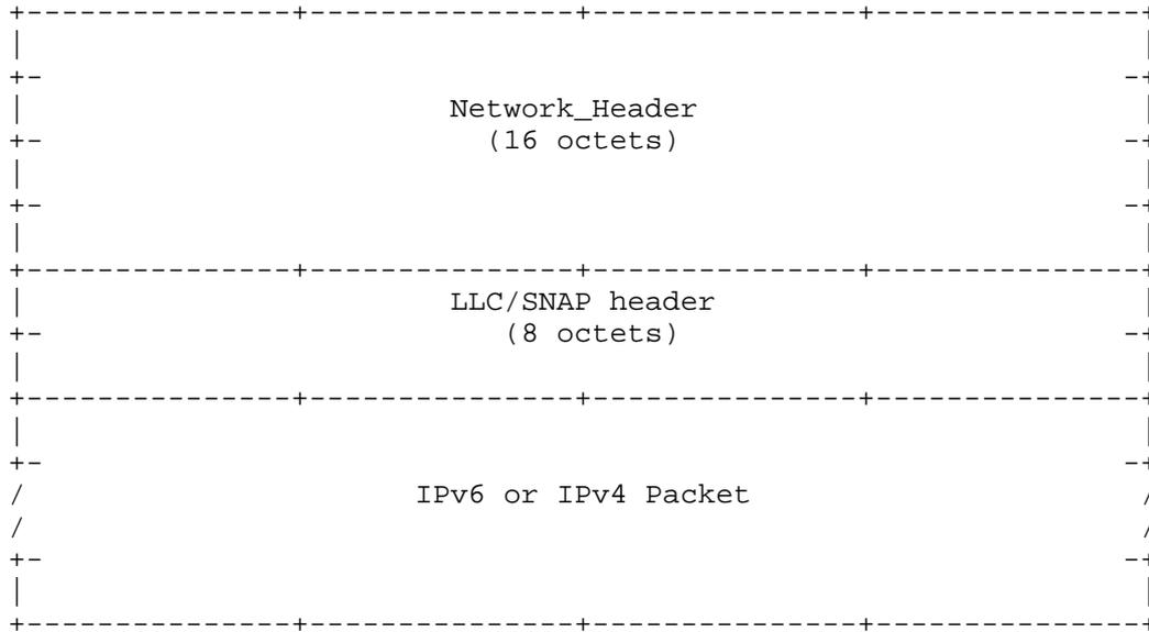
Figure 2: FC Information Unit Mapping an IP Packet
