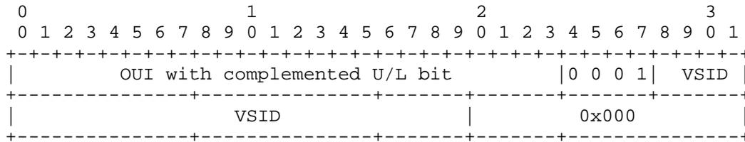
Figure 9: EUI-64 Address from a Format 0x1 Name\_Identifier
