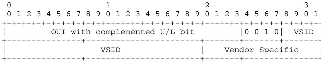
Figure 12: EUI-64 Address from a Format 0x2 Name\_Identifier
