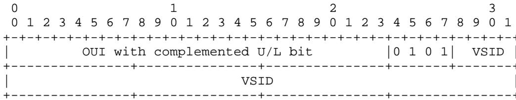
Figure 15: EUI-64 Address from a Format 0x5 Name\_Identifier
