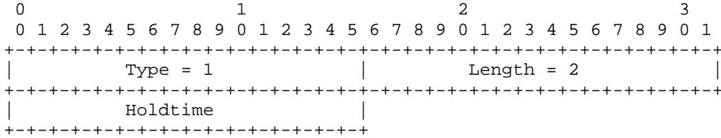
Holdtime is the amount of time a receiver must keep the neighbor reachable, in seconds. If the Holdtime is set to '0xffff', the receiver of this message never times out the neighbor. This may be used with dial-on-demand links, to avoid keeping the link up with periodic Hello messages.
