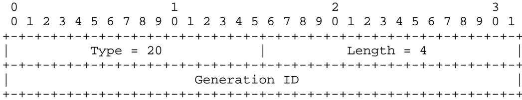
Generation ID is a random 32-bit value for the interface on which the Hello message is sent. The Generation ID is regenerated whenever PIM forwarding is started or restarted on the interface.
