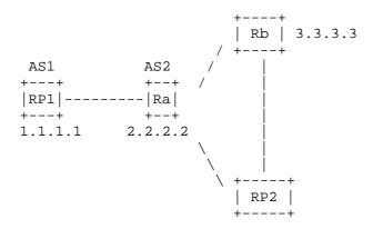
where RP2 MSDP and MBGP peers with Ra (using 2.2.2.2) and with Rb (using 3.3.3.3). When the MSDP SA update arrives on RP2 from Ra, the MSDP RPF check for 1.1.1.1 passes because RP2 receives the SA update from MSDP peer 2.2.2.2, which is also the correct MBGP next hop for 1.1.1.1.
