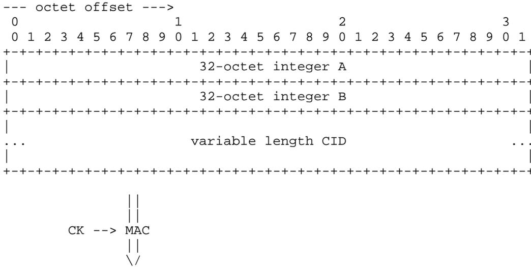
Figure 6: Example Encoding of PAX\_STD-2 MAC Data
