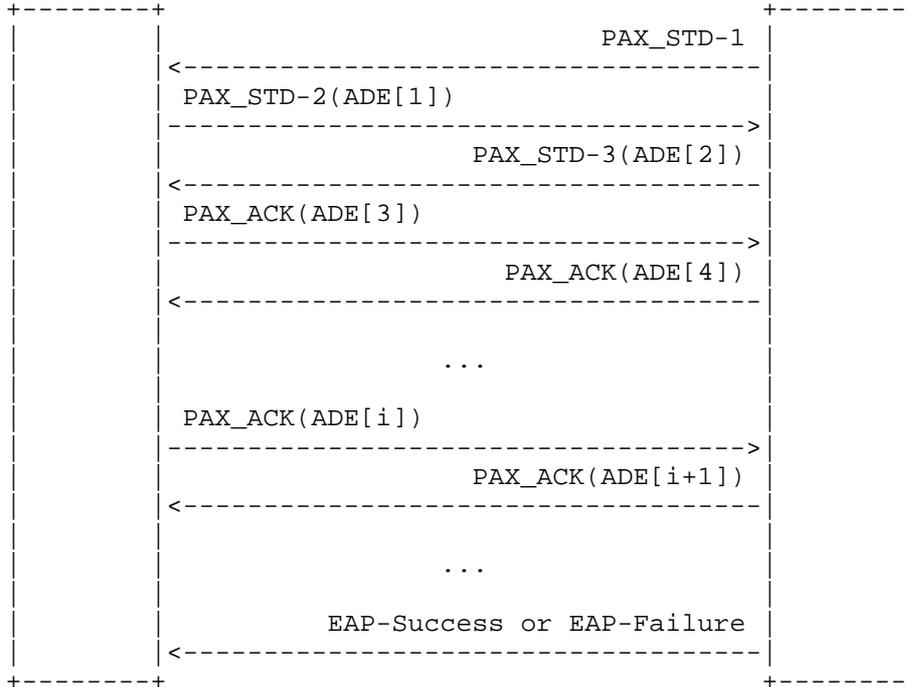
Figure 3: Extended Diagram of EAP-PAX Packet Exchanges
