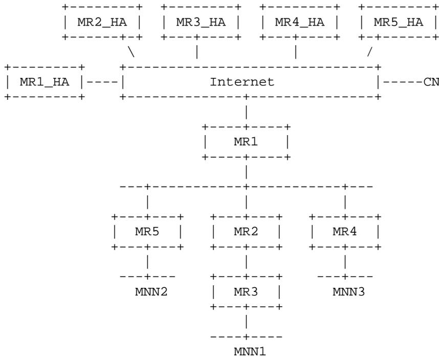
Figure 3: An Example of a Nested Mobile Network
