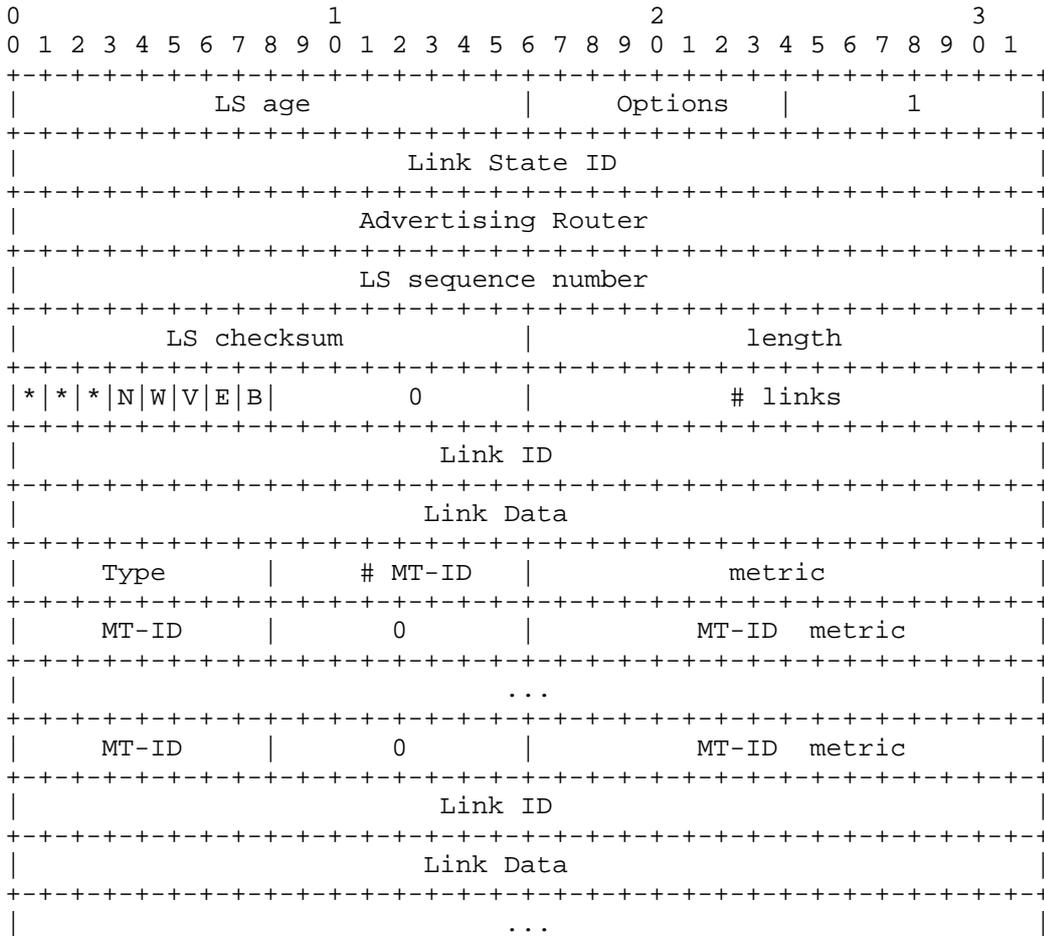
Figure 2: Router-LSA Format
