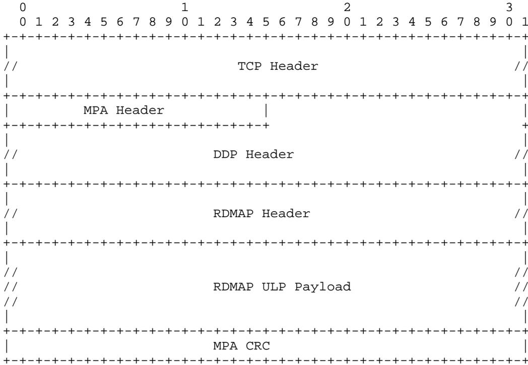
Figure 2: MPA, DDP, and RDMAP Header Alignment
