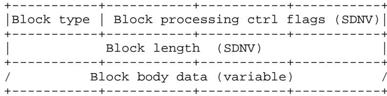
Figure 6: Block Layout without EID Reference List
