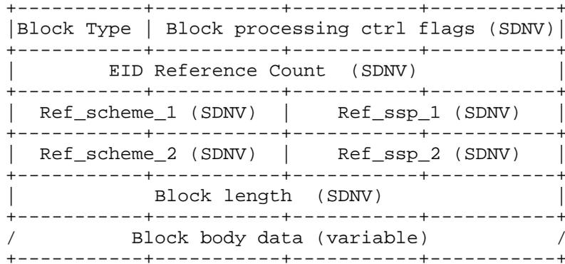
Figure 7: Block Layout Showing Two EID References
