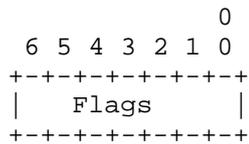
Figure 4: Block Processing Control Flags Bit Layout
