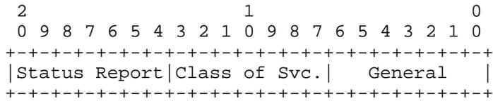
Figure 3: Bundle Processing Control Flags Bit Layout
