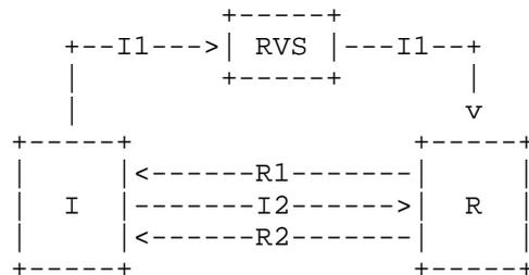
Figure 2: HIP base exchange with a rendezvous server.
