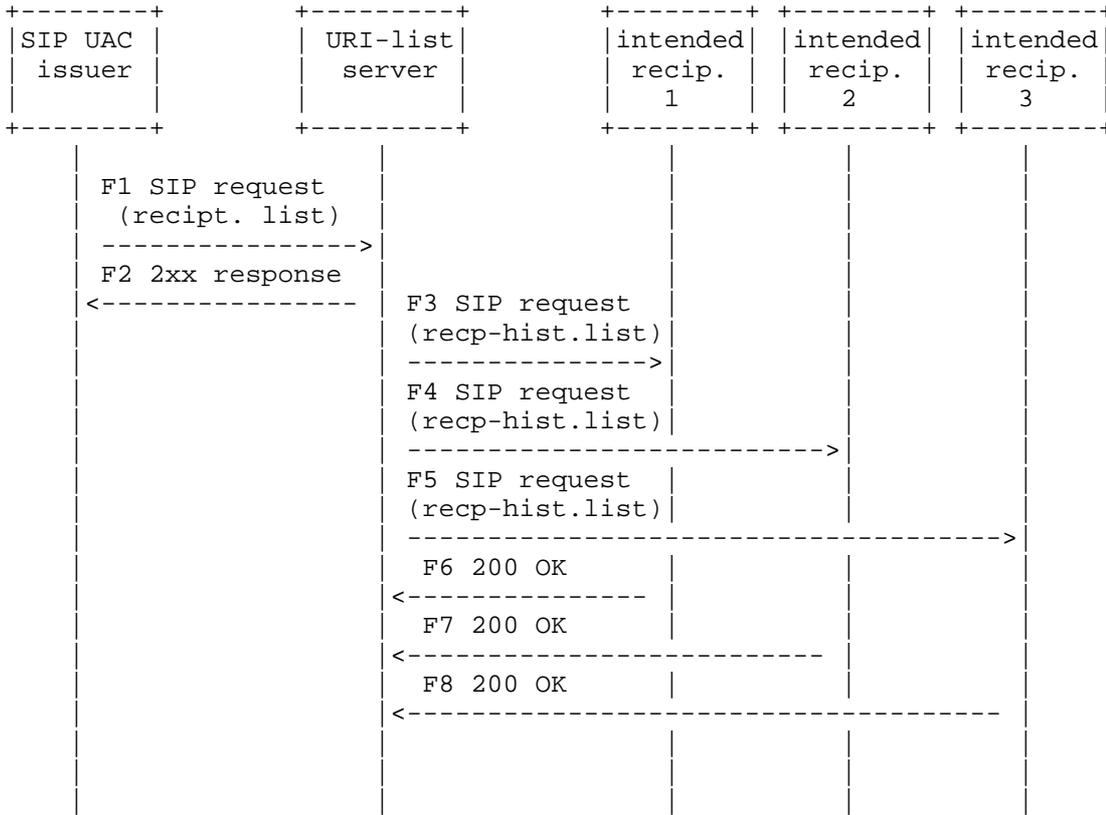
Figure 1: Example of operation
