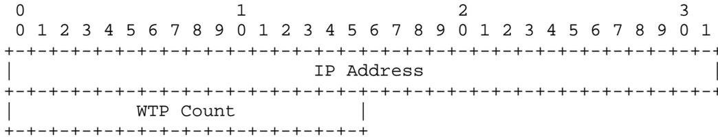
Type: 10 for CAPWAP Control IPv4 Address
