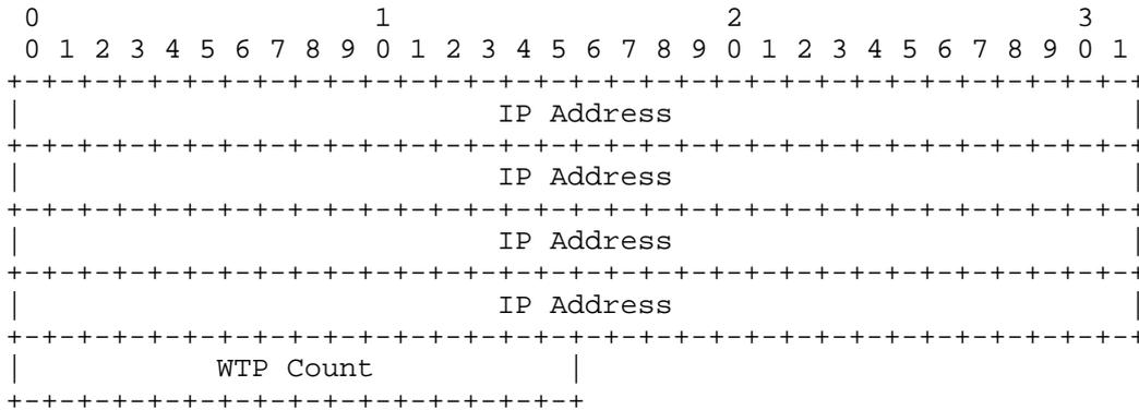
Type: 11 for CAPWAP Control IPv6 Address
