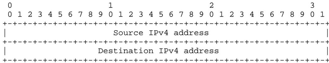
Figure 12: END-POINTS Object Body Format for IPv4
