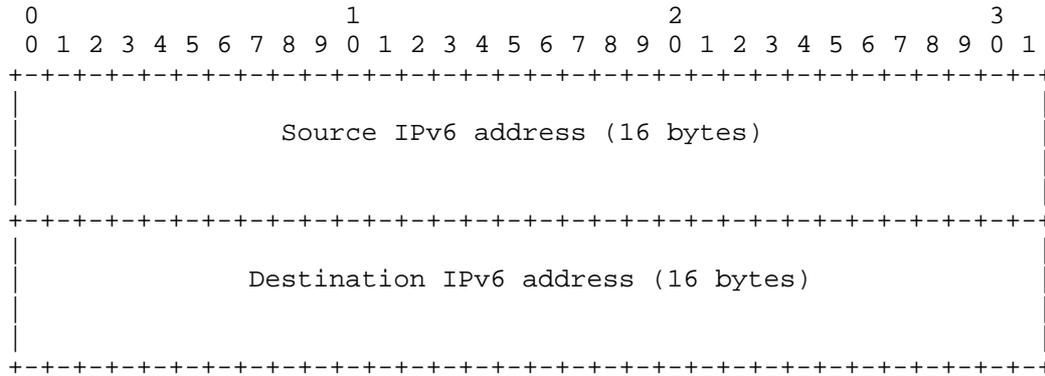
Figure 13: END-POINTS Object Body Format for IPv6
