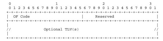
OF Code (2 bytes): The identifier of the objective function. IANA manages the "PCE Objective Function" code point registry (see Section 6).
