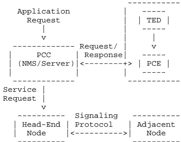
Figure 1: PCE-Based Architecture for Global Concurrent Optimization
