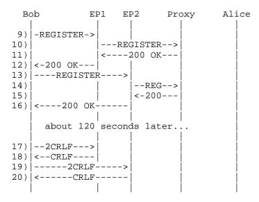
In message #9, Bob's UA sends its first registration through the first edge proxy in the outbound-proxy-set by including a loose route. The UA includes an instance-id and reg-id in its Contact header field value. Note the option-tags in the Supported header.
