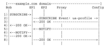
In this example, the DNS server happens to be configured so that sip: example.com resolves to EP1 and EP2.
