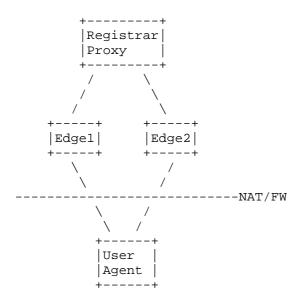
The edge proxy includes a Path header [RFC3327] so that when the proxy/registrar later forwards a request to this UA, the request is routed through the edge proxy.
