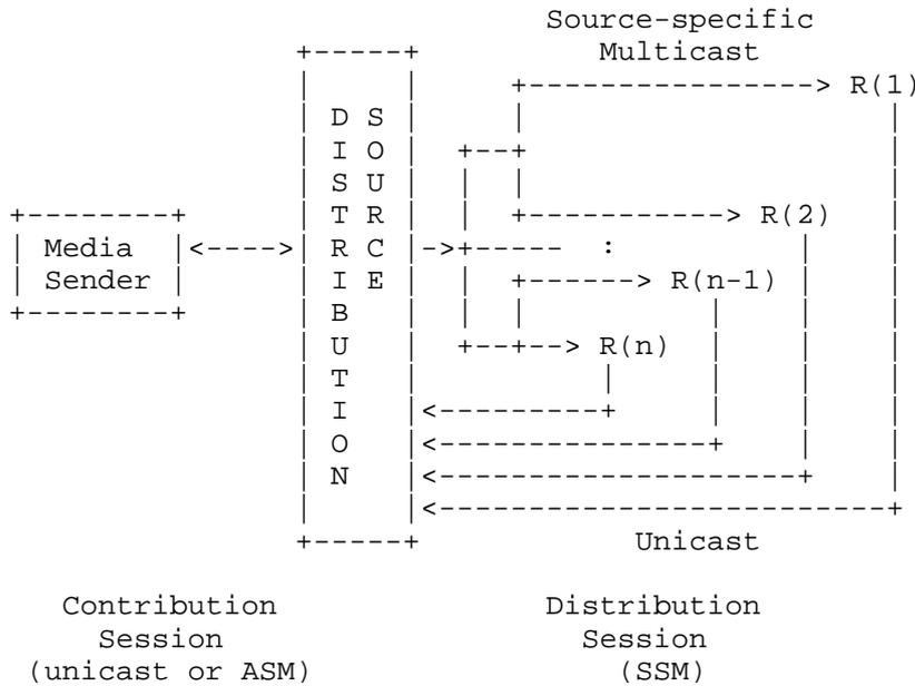
Figure 4: One Media Sender Separate from Distribution Source
