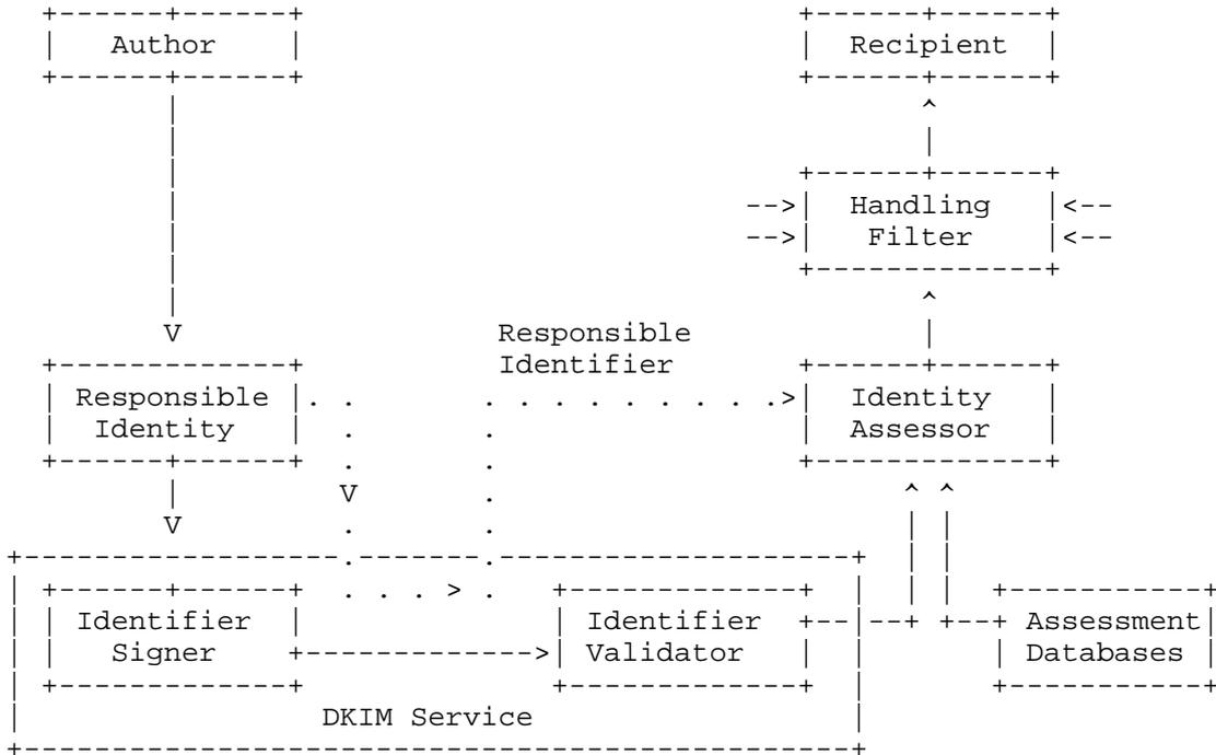
Figure 1: Actors in a Trust Sequence Using DKIM
