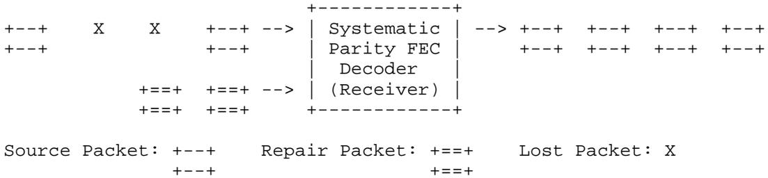
Figure 2: Block diagram for systematic parity FEC decoder
