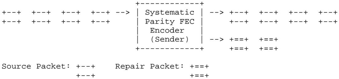
Figure 1: Block diagram for systematic parity FEC encoder
