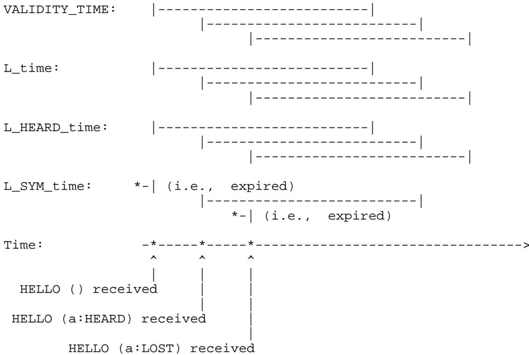
Figure 8: HELLO Message Processing: Network Address Lost
