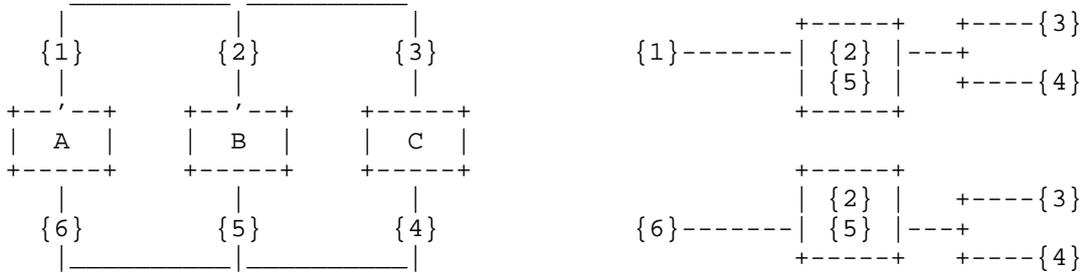
Figure 20: Single Addresses, with All Routers Having Two Interfaces (Left), and Corresponding NHDP Representation (Right)
