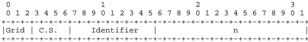
The structure of the label in the case of CWDM is the same as that of the DWDM case.
