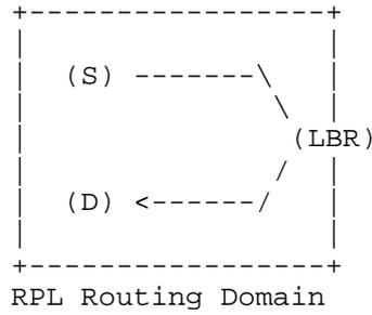
In the above scenario, datagrams travel from S to D through the Low-Power and Lossy Network Border Router (LBR). Between S and the LBR, the datagrams are routed using the DAG built by the RPL and do not contain an SRH. The LBR encapsulates received datagrams unmodified using IPv6-in-IPv6 and the SRH is included in the outer IPv6 header.
