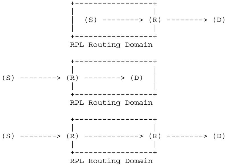
In the scenarios above, R may indicate a RPL Border Router (when connecting to other routing domains) or a RPL Router (when connecting to hosts). The datagrams have the following structure when traveling within the RPL routing domain:
