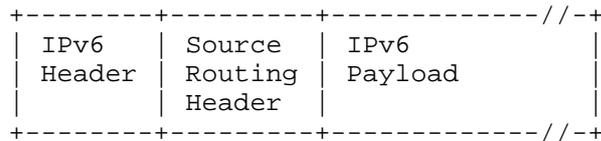
S's address is carried in the IPv6 header's Source Address field.
