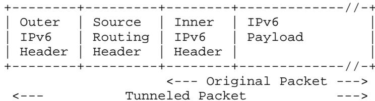
Note that the outer header (including the SRH) is added and removed by the RPL router.
