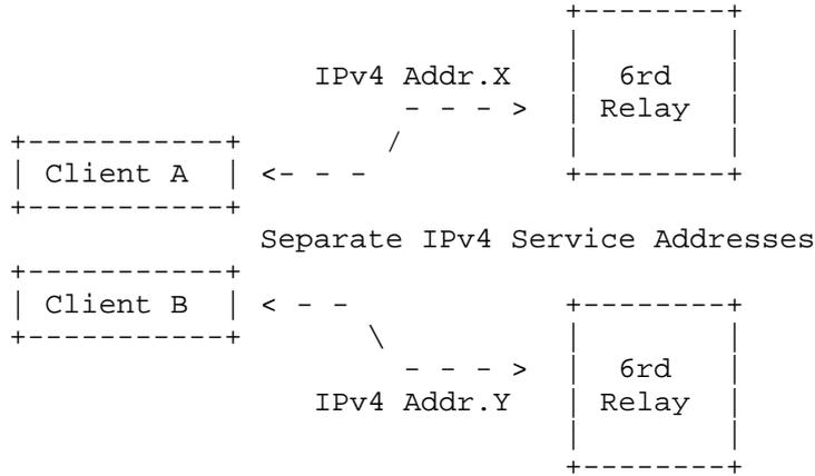
Figure 2: 6rd Multiple IPv4 Service Address Model
