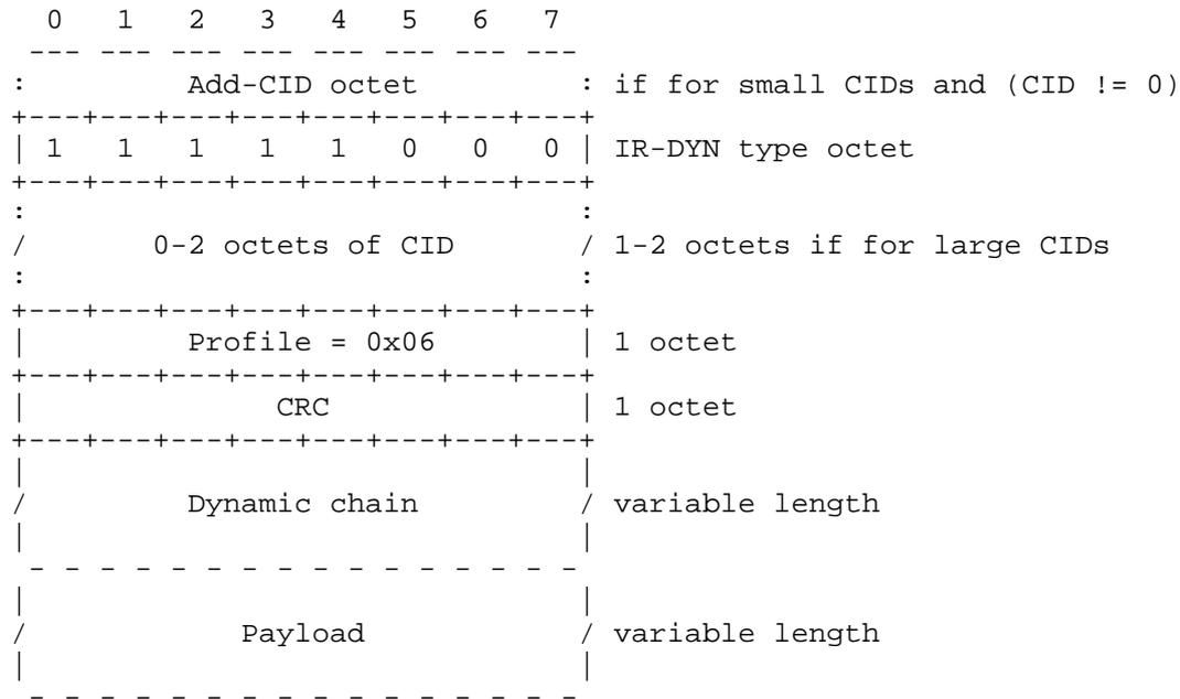
CRC: 8-bit CRC, computed according to Section 5.3.1.1 of [RFC5795]. The CRC covers the entire IR-DYN header, thus excluding payload, padding, and feedback, if any.
