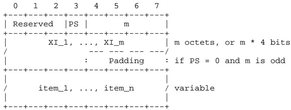
Reserved: MUST be set to zero; otherwise, the decompressor MUST discard the packet.
