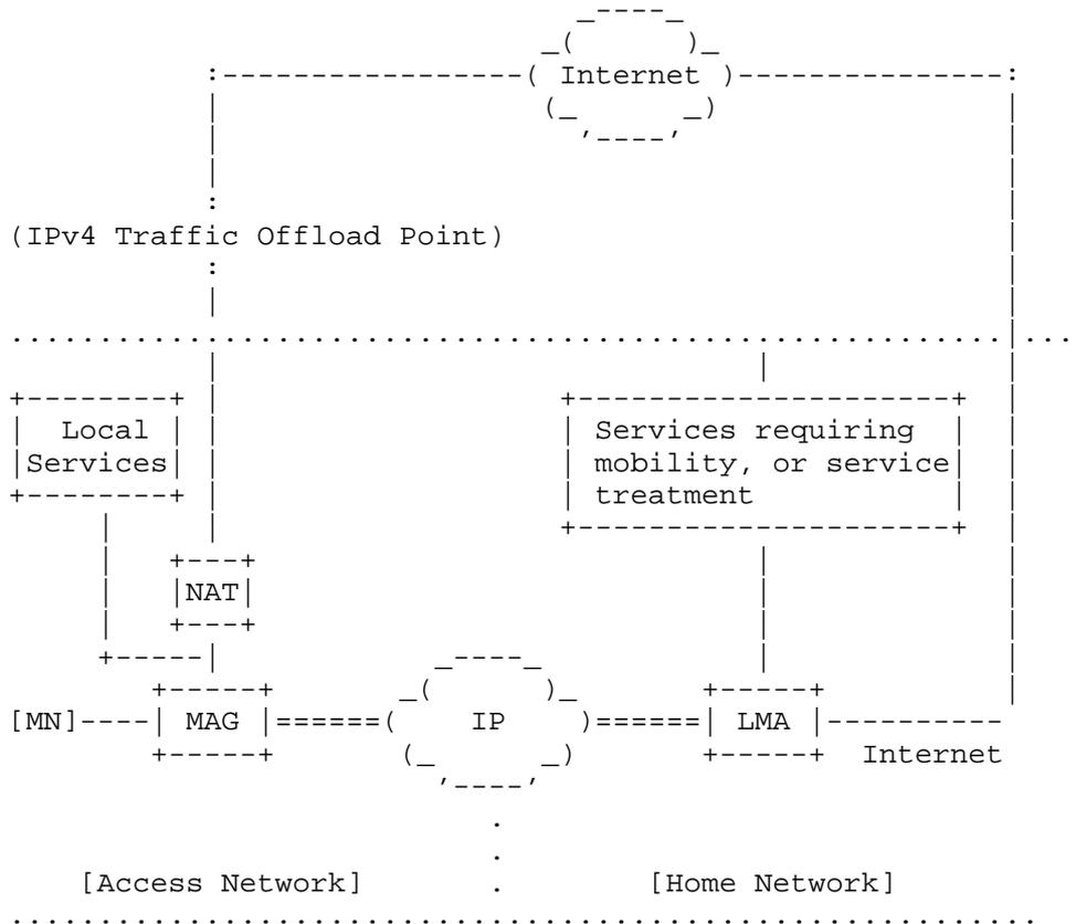
Figure 1: IPv4 Traffic Offload Support at the MAG
