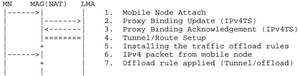
Figure 2: Exchange of IPv4 Traffic Offload Selectors
